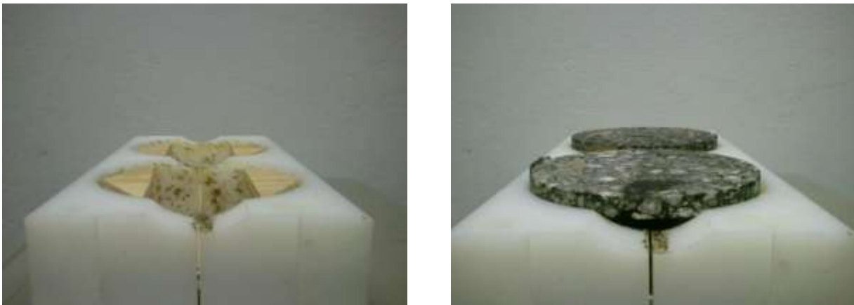
Figure 20. Support installed in mold with and without practice sample placed on top (side view)
