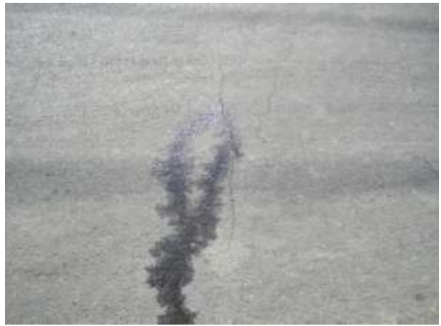
d. water couldn't penetrate the crack
